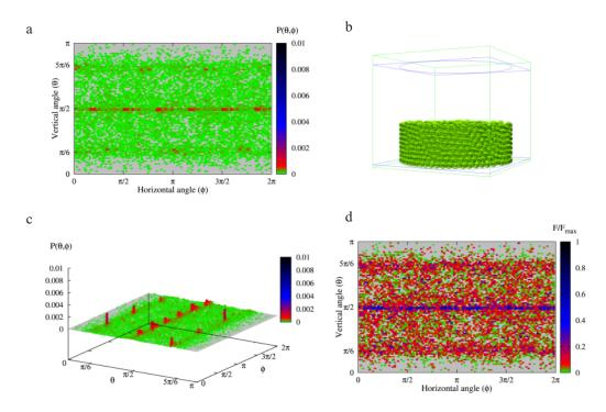
**Fig. 8.** Characteristics of the structure of the assembly of spherical particles formed in the cylindrical container by disperse filling: a – planar projection of the distribution of the contact points, b – a 3D view of the assembly, c – distribution of the contact points – a 3D view, d – distribution of normalized values of the contact forces.
