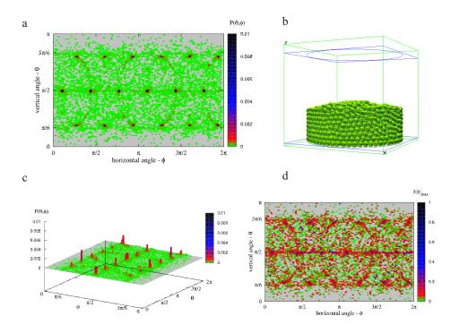
**Fig. 6.** Characteristics of the structure of the assembly of spherical particles formed in the cylindrical container by centric filling: a - planar projection of the distribution of the contact points, b - a 3D view of the assembly, c - distribution of the contact points - a 3D view, d - distribution of normalized values of the contact forces.
