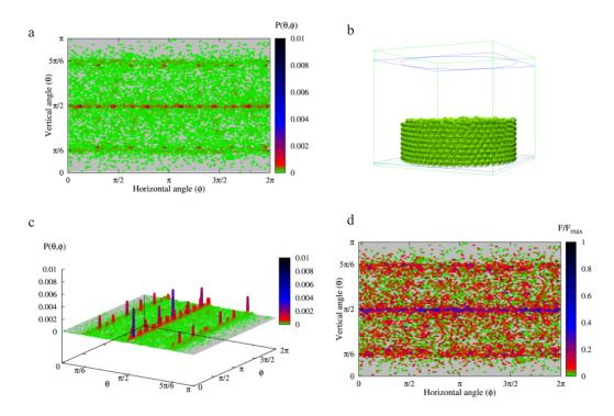
**Fig. 7.** Characteristics of the structure of the assembly of spherical particles formed cylindrical container by in-volume filling: a - planar projection of the distribution of the contact points, b - a 3D view of the assembly, c - distribution of the contact points - a 3D view, <math>d - distribution of normalized values of the contact forces.
