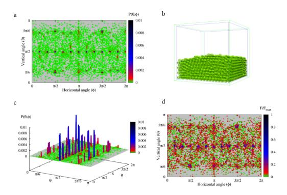
**Fig. 4.** Characteristics of the structure of the assembly of spherical particles formed in cuboidal container by centric filling: a - planar projection of the distribution of the contact points, b - a 3D view of the assembly, c - distribution of the contact points - a 3D view, d - distribution of normalized values of the contact forces.
