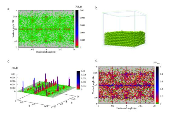
**Fig. 5.** Characteristics of the structure of the assembly of spherical particles formed in the in-volume filled cuboidal container: a - planar projection of the distribution of the contact points, b - a 3D view of the assembly, c - distribution of the contact points - a 3D view, <math>d - distribution of normalized values of the contact forces.
